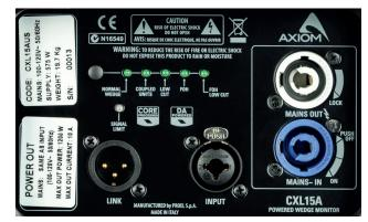
compression driver. Input and link connections are via balanced 3-pin XLR connectors, and a ground lift switch is provided for humfree operation. Mains power is connected through a locking Neutrik<sup>®</sup> powerCON<sup>™</sup>, and a power out connector allows mains power to be linked to additional CXL12A cabinets.
